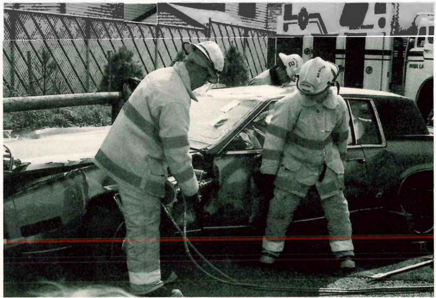
*The Heavy Rescue Squad uses its skill and a specialized hydraulic tool to demonstrate an automobile extrication procedure at a public safety demonstration in town.*
